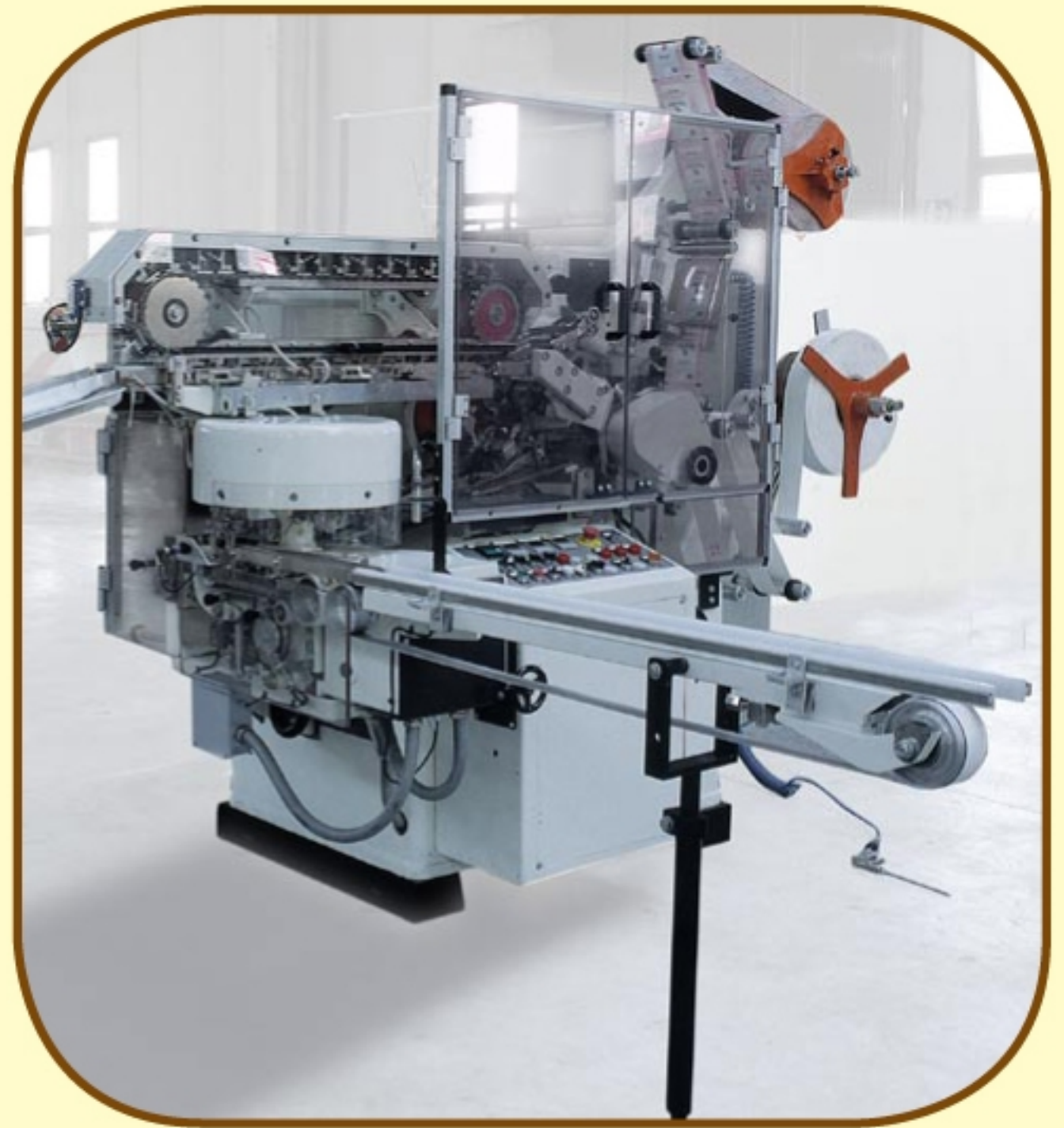
Rebuilt Carle & Montanari Wrapper
